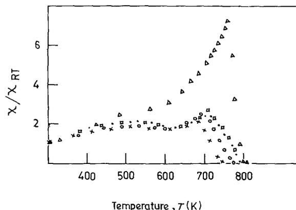
Figure 2 The temperature dependence of relative a.c. susceptibility ( $\chi/\chi_{RT}$ ) at low field for the  $\text{Ca}_x\text{Co}_{1-x}\text{Fe}_2\text{O}_4$  system for  $x = (\Delta) 0.05, (\times) 0.2, (\circ) 0.3, (\bullet) 0.6$  and  $(\square) 0.8$ .
