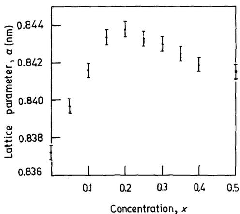
Figure 1 Variation of the lattice constant (cubic phase) of the  $\text{Ca}_x\text{Co}_{1-x}\text{Fe}_2\text{O}_4$  system as a function of concentration ( $x$ ), for  $x \leq 0.5$ .
