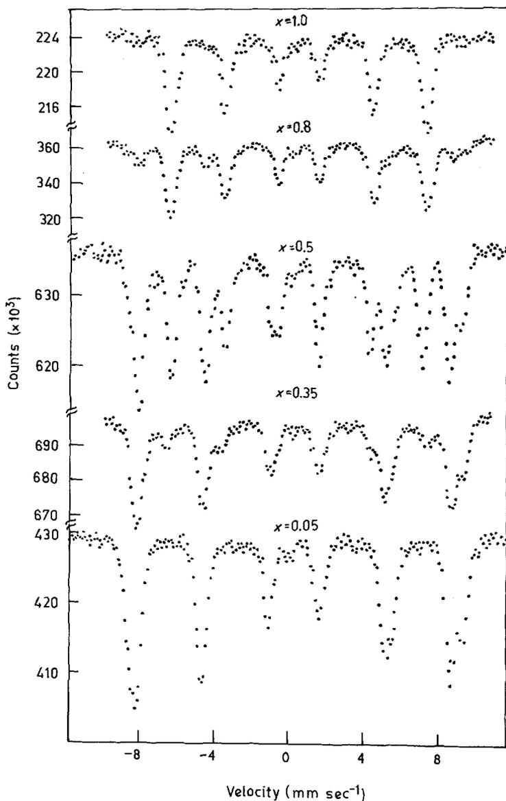
Figure 4 Mössbauer spectra of the  $\text{Ca}_x\text{Co}_{1-x}\text{Fe}_2\text{O}_4$  system at 77 K for  $x = 0.05, 0.35, 0.5, 0.8$  and 1.0.
