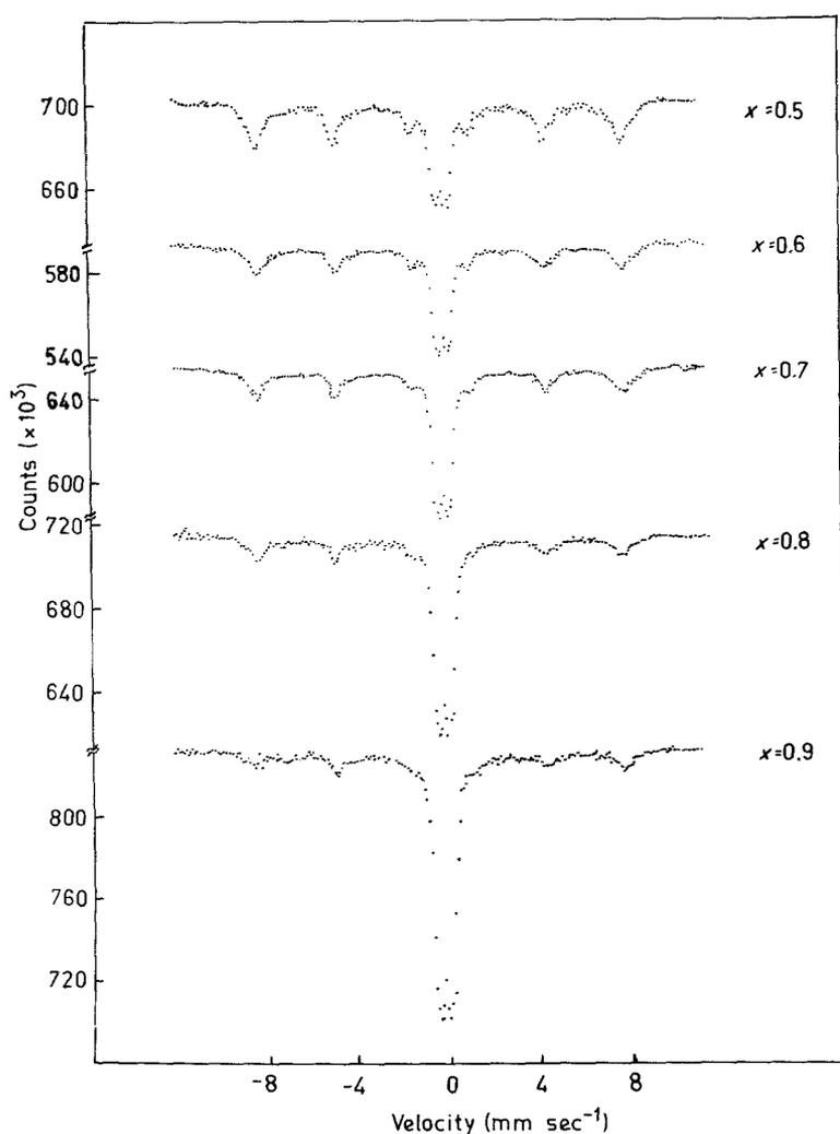
Figure 3 Room-temperature (300 K) Mössbauer spectra of the  $\text{Ca}_x\text{Co}_{1-x}\text{Fe}_2\text{O}_4$  system for  $x = 0.5, 0.6, 0.7, 0.8$  and  $0.9$ .
